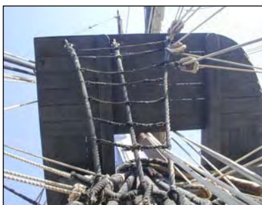
After Climbing 60 feet up the main shrouds, you have to climb up 6 feet of futtock shrouds, hanging on backwards for dear life.
